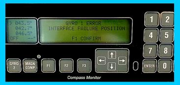
Gyrocompass: Alarm, and drifts over time
